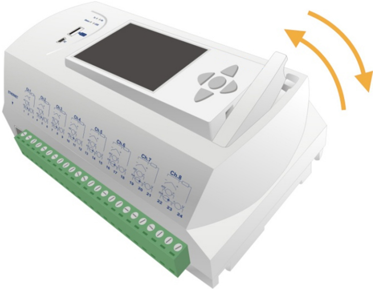
Fig. 10 – Attaching and detaching the Data Logger DISPLAY
