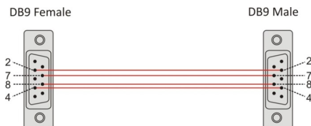
Figure 27 – Building an extension cable
